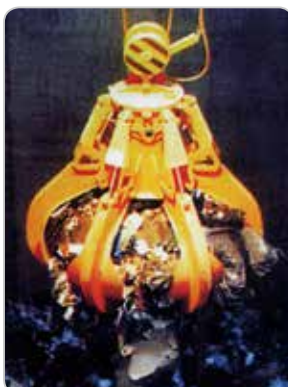
可自动操作的电动液压垃圾抓斗 Can be automated electro-hydraulic pull
